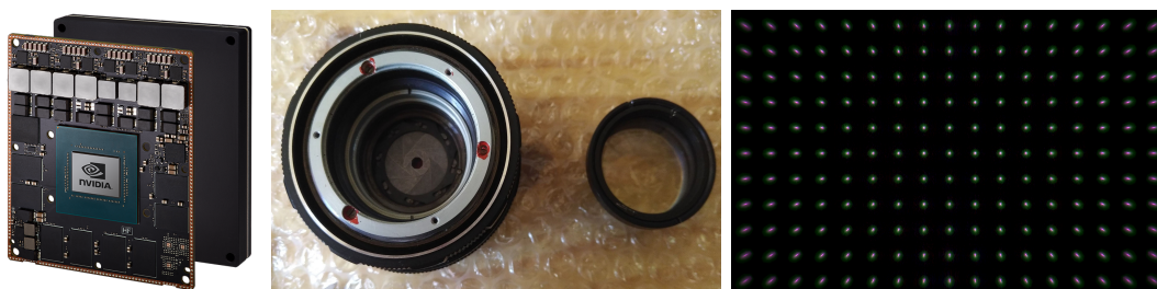
Figure 1: Left: the Nvidia Jetson Xavier. Center: the custom lens. Right: the field of point spread functions describing the blur induced by the lens at different locations.
